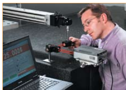
CMM calibration using an XL-80 laser
