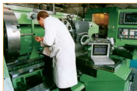
Checking lathe performance with a Renishaw ballbar
