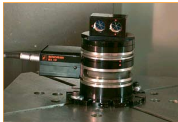
RX10 showing fixing to table and angular reflector
