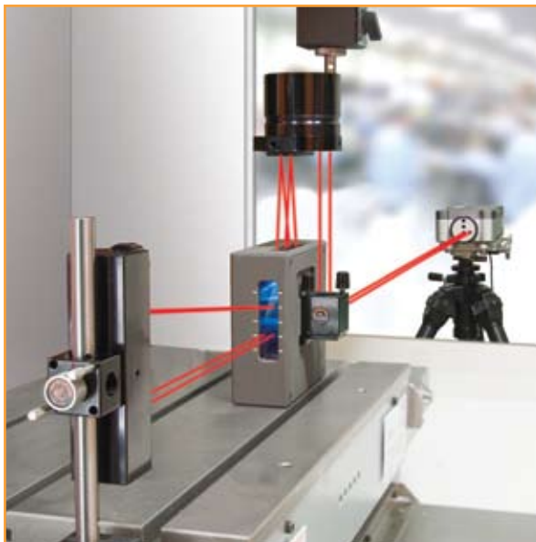
X-Z axis squareness measurement on a VMC
